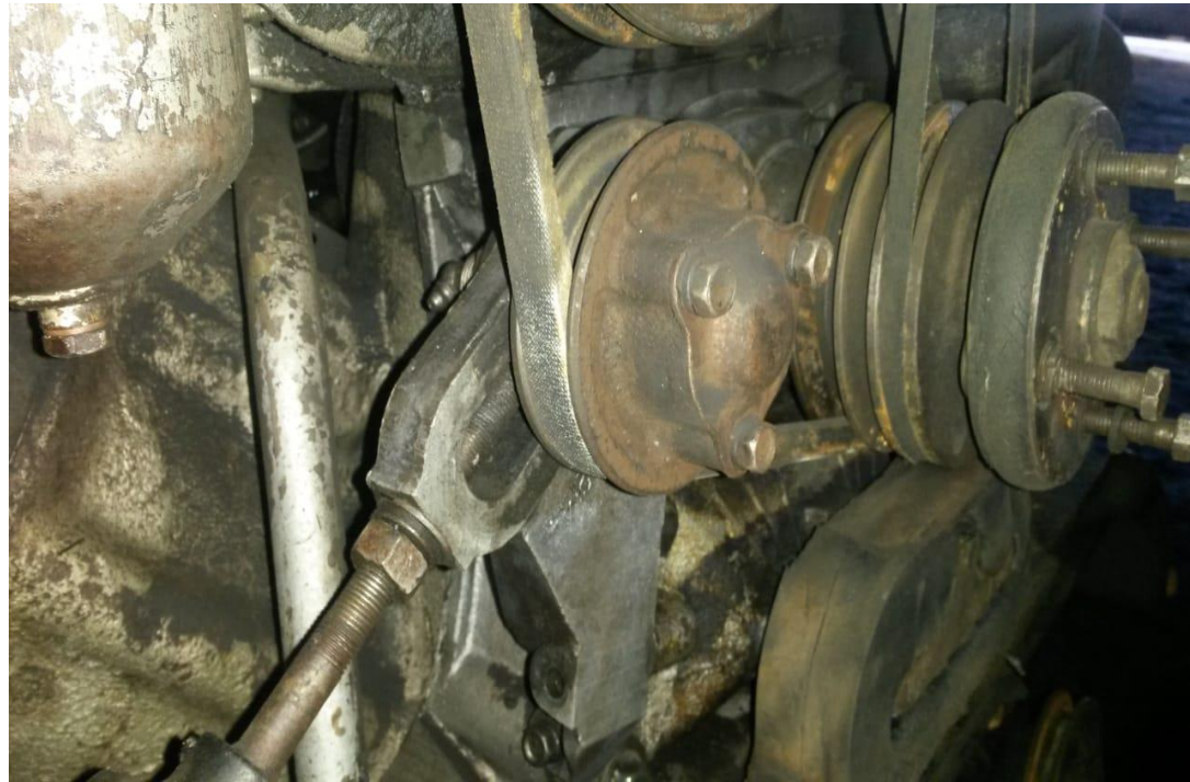
Type of oil pump drive on the car engine
