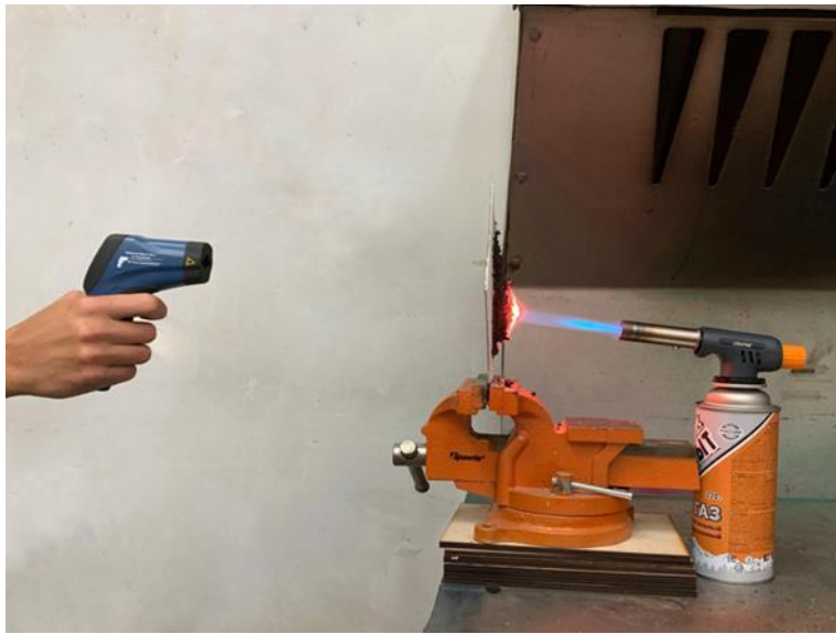
Fig. 1. Conducting exposed to open flame temperature measurement samples.
